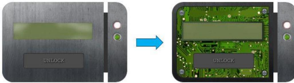
FIGURE 47: REMOVE THE LOCK'S COVER TO REVEAL THE PRINT CIRCUIT
